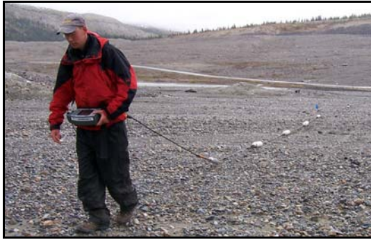
Figure 2. Person pulling the OhmMapper on the outwash plain.
